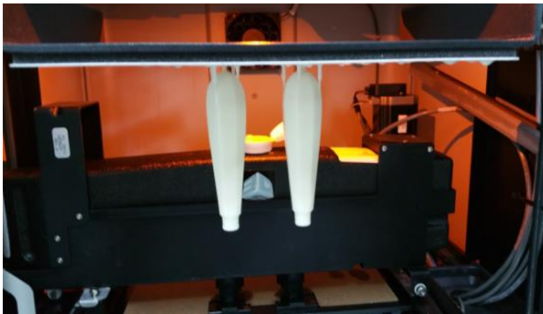
Fig. 2. Elevator handle prototypes obtained by stereolithography technology on PROJET 1500
