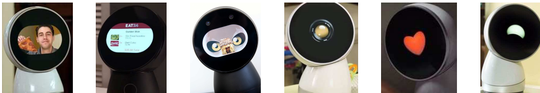
Figure 6: Different functions of Jibo's screen. From left to right, Jibo's screen is used to display the stream of a videoconference, a graphical user interface, an illustration of children's story, an icon indicating the current application, an icon expressing an emotion and a facial expression.
