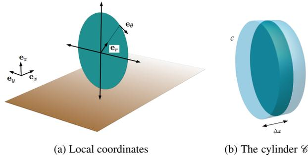
Fig. 1.9: (a) The local reference frame at the actuator disc of the turbine, using cylindrical coordinates; (b) The cylinder  $\mathcal{C}$  that extends the actuator disc. Mill forces are applied to particles that lie inside.
