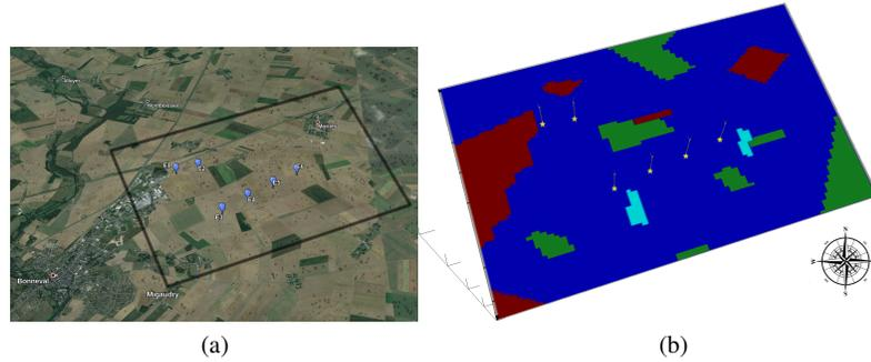
Fig. 1.10: (a) Aerial view of the “Parc de Bonneval” from Google-Earth; (b) Aerial view of the simulated wind farm. The pattern defines the roughness length. Blue part represents farmland (0.04 m), red are small town (0.4 m), green are uncut grass (0.01 m), cyan are small forest (0.15 m). Yellow stars represent the turbines.
