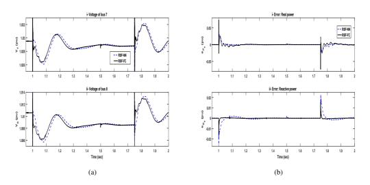
**Figure 4.** Control response to step changes in real and reactive powers of the transmission line under online variation of  $R_s$  (up to  $\pm 40\%$ ) and online variation of  $X_s$  (up to  $\pm 20\%$ ). (a) Voltage of bus 7 and 8. (b) Error on real power and reactive power
