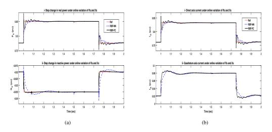
**Figure 3.** Control response to step changes in real and reactive powers of the transmission line under online variation of  $R_s$  (up to +40%) and online variation of  $X_s$  (up to +20%). (a) Active and reactive power in the transmission line. (b) DQ currents
