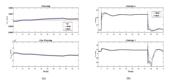
**Figure 5.** Control response to step changes in real and reactive powers of the transmission line under online variation of  $R_s$  (up to  $\pm 40\%$ ) and online variation of  $X_s$  (up to  $\pm 20\%$ ). (a) DC bus voltage of SSSC. (b) Control input of SSSC
