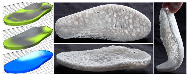
Figure 23: A 3D printed shoe sole. Left : Control fields used on the model, density (top), orthotropy strength (middle) and angle (bottom). Right : Printed shoe, top, side and bending. The shoe is printed without any skin to reveal the foam structure.
