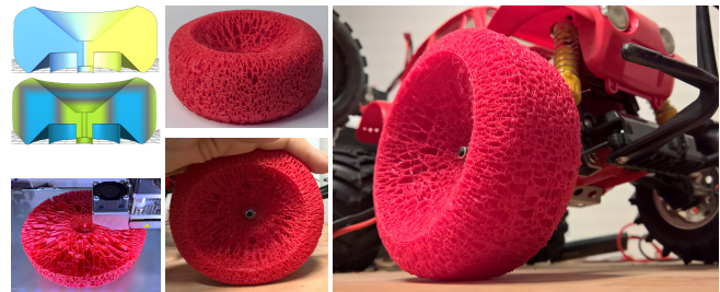
Fig. 22. Top left: Orientation field \zeta (top) and density field (below). The anisotropy is constant at \sigma = 0.3 . Bottom left: Wheel being printed on an Ultimaker 2 with Semiflex filament at 0.3 mm thickness. The print took 19 hours. Middle column: The finished wheel and its deformation under load. Right: Ready to run!
