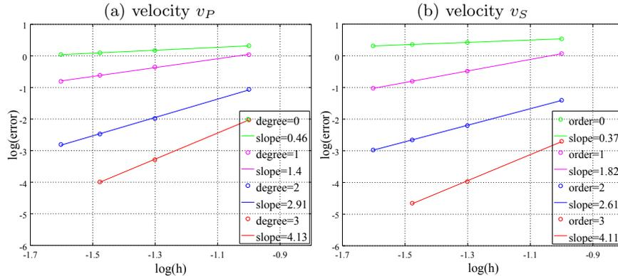
Even though the initial model is limited (large mesh of  $30 \times 30 \times 30$  elements, Dirichlet boundaries, which causes many reflections), the numerics reproduce the expected propagation characteristics quite well, and the convergence in both cases is of order higher than the corresponding approximation order.
