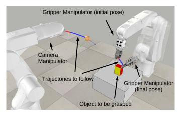
Fig. 1. the experimental setups showing the two 6-dof serial manipulator arms equipped with a camera and a gripper, respectively, together with the object to be grasped.
