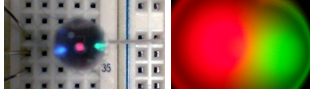
Figure 3. The RGB LED without modulation. On the left, the LED is strongly dimmed with the 3 channels ON. On the right, the LED is normally dimmed with only the red and green channel ON.
