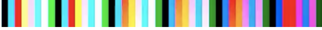
Figure 2. The same 8-CSK symbols sent consecutively and repetitively are perceived differently in the picture.
