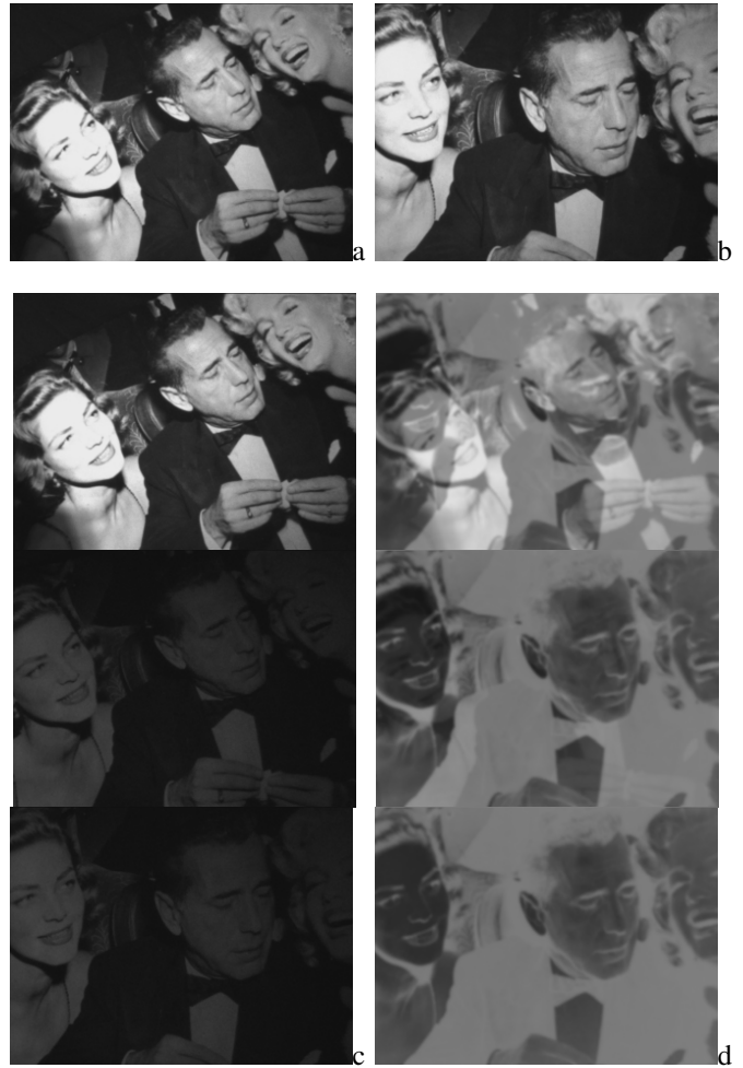
Fig. 6. ZNCC based visual servoing with important lighting variations (a-b) initial and desired image acquired by the camera. (c-d) images acquired during the positioning task (iteration 1, 75 and 1000) and the corresponding error
