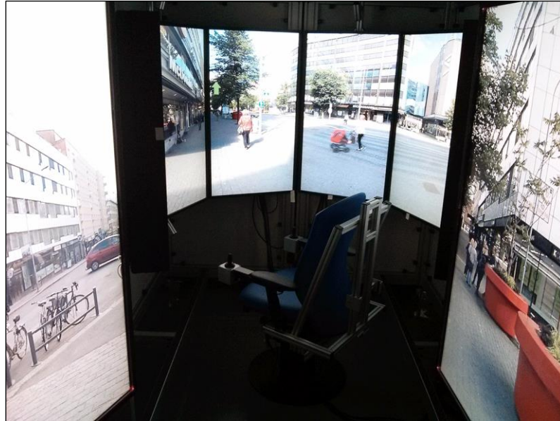
Fig. 1. The cCAVE system. The rotating chair used for interaction is at the center of the system. Eight monitors (only 6 shown in the image) each show 45 degrees of the omnidirectional video content. The two monitors in front are attached to the doors that are opened for entrance and closed during use.
