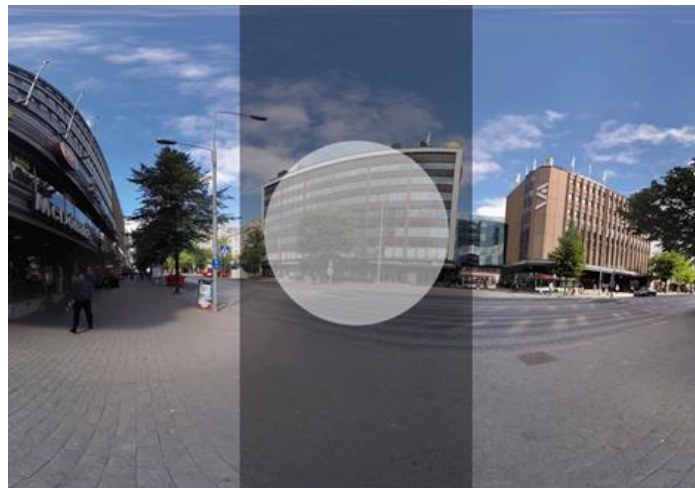
Fig. 3. The hotspot activation sectors illustrated in both applications. The gray coordinate area represents the coordinate range of hotspots in cCAVE, and the circular area represents the X- and Y- coordinate range used in Amaze360.
