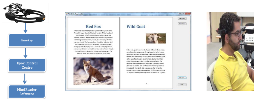
Figure 1: (left) Key components to operate MindReader system (centre) MindReader beta version (right) User interacting with MindReader
