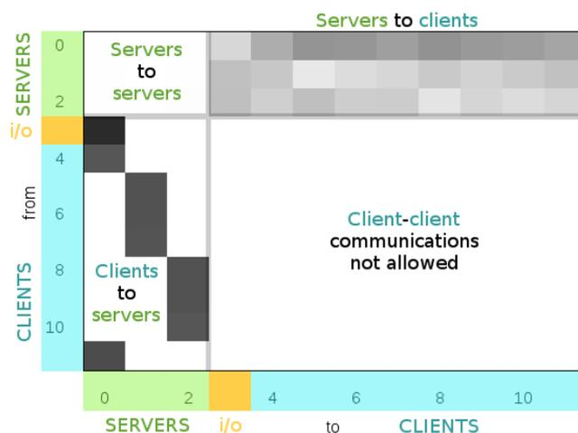
Fig. 7: **Topology E**. Communication heatmap. Each cell represents the cumulative size of messages that have been sent *from* tasks indexed vertically, *to* tasks indexed horizontally. Tasks 0 to 2 are memory servers. Task 3 is the i/o client. Tasks 4 to 11 are processing tasks. Values are normalized to grayscale, darker is bigger.
