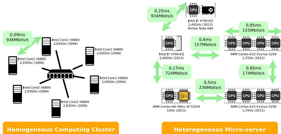
Fig. 2: Testbeds used for the experimentations: an homogeneous cluster of desktop computers and an heterogeneous Christmann RECS 3 Antares Box Microserver. Latencies are given by *Ping* and throughputs by *Iperf*. If not specified, we assume roughly the same performances as similar links.
