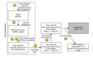
Fig. 2. Threat modelling and security testing steps
