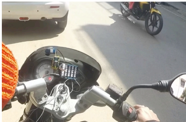
Figure 4: Riding with the ReRide display positioned as part of the existing dashboard
