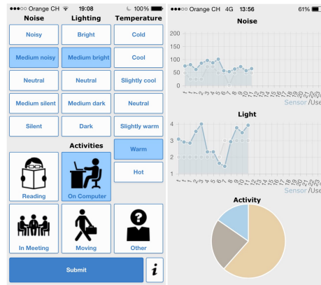
Fig. 5. Through simple user questionnaires following the experience sampling approach, users' comfort perception is compared with smartphone sensor data.
