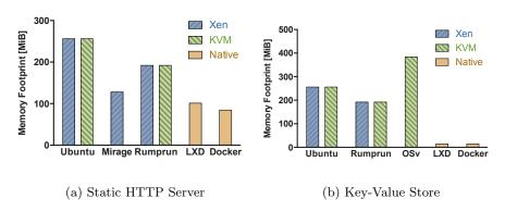
Fig. 5. The memory footprints of the static HTTP server scenario (a) and the Key-Value Store scenario (b) were measured for each virtualization technique.
