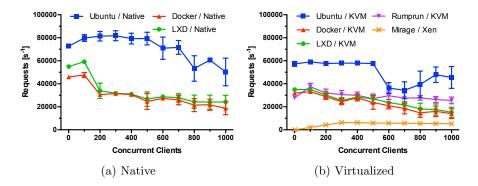
**Fig. 4.** Throughput of *Nginx* (1.8.0) was evaluated on native hardware (a) and in virtualized environments (b). For MirageOS, the *conduit server* was used. Throughput was measured using *weightttp* and the modified *abc wrapper* utility.
