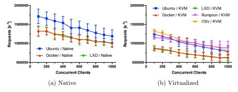
**Fig. 6.** Throughput of *Redis* (version 3.0.1) was evaluated on native hardware (a) and in virtualized environments (b). The plotted values show the throughput for GET requests as retrieved through the *redis-benchmark* utility.
