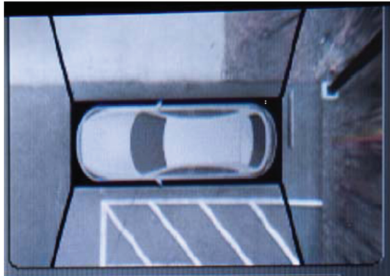
Figure 9.7 Top view of a parking assistance system.
