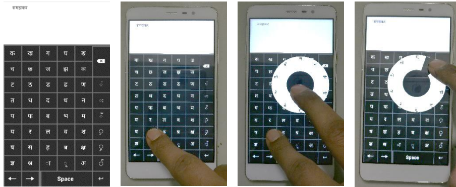
Fig. 4a accessible version of Swarachakra , Fig. 4b explore by touch to locate key, Fig. 4c second-finger tap to activate chakra , Fig. 4d lift the first finger and slide the second finger to make a selection
