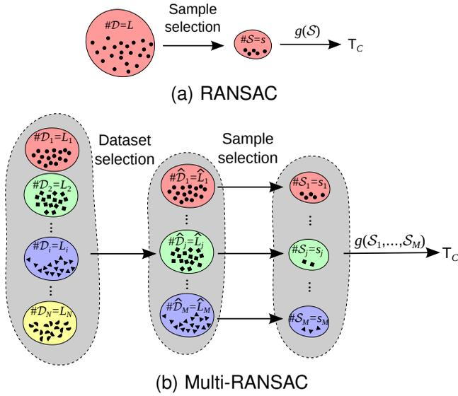
Fig. 5. Generation of candidate models  $T_C$ . (a) In each RANSAC iteration a subset  $S$  with  $s$  samples is selected from dataset  $D$ . (b) In each multi-RANSAC iteration there are two sampling steps: the first step randomly selects  $M$  of the  $N$  datasets  $D_1, \dots, D_N$ ; in the second step  $s_j$  samples are selected from each of the  $M$  selected datasets  $\hat{D}_j$ .
