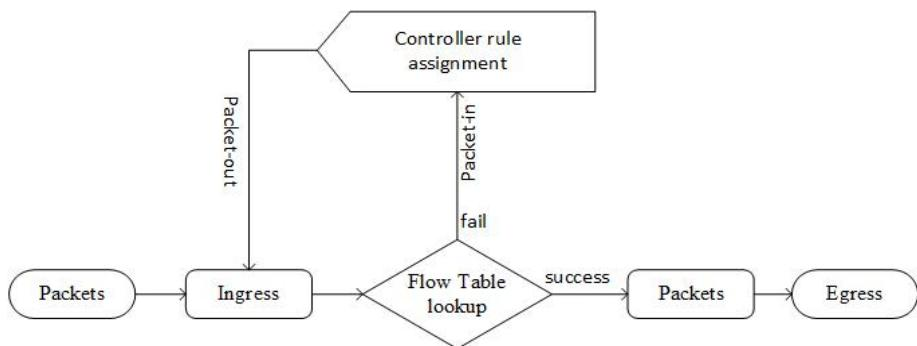
**Fig. 2.** The packet forwarding of an OpenFlow switch.
