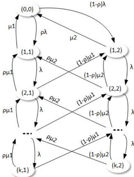
**Fig. 9.** State transition diagram of an M/H2/1 queue
