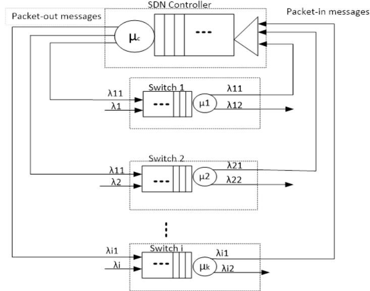
**Fig. 8.** OpenFlow-based SDN queueing model
