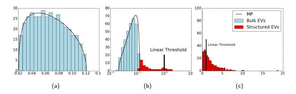
Fig. 8: (a) Singular values distribution of the initial random matrix compared to Marchenko-Pastur law. (b) With the training we can see some singular values strengthening and overcoming the threshold set by the Marchenko-Pastur law. (c) Distribution of the singular values after a long training: we can see many outliers spread above threshold and a spike of below-threshold singular values near zero.
