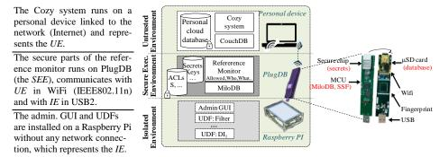
Fig. 2. Experiment platform: software and hardware (right).
