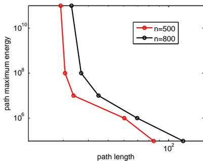
Figure 9: Path maximum energy versus hops  $d_m = 3.3, d_r = 2.3$
