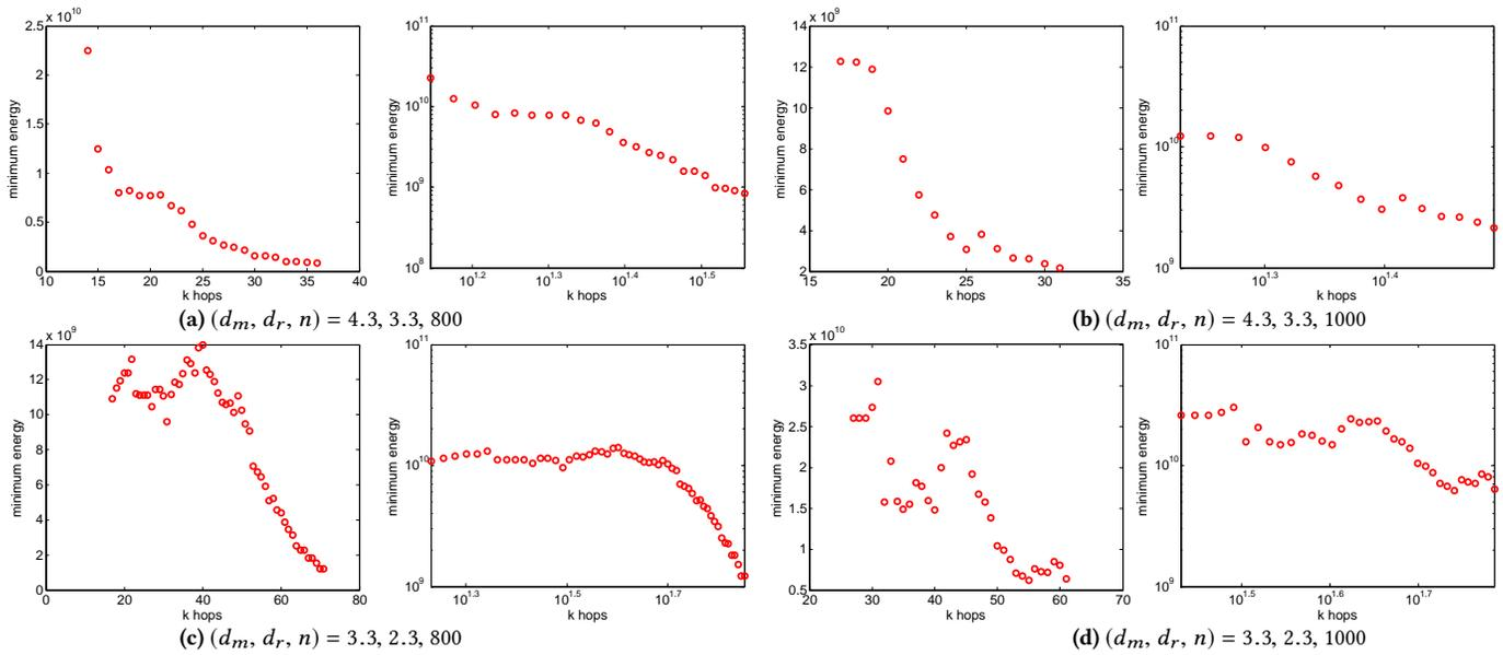
Figure 7: Minimum cumulated end-to-end energy versus hops, averaging over 100 transmitter-receiver pairs,  $\delta = 4$ , linear scale left side of sub-figures, logarithmic scale right side of sub-figures
