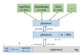
Figure 3: Constructing a TLS 1.3 record fragment
