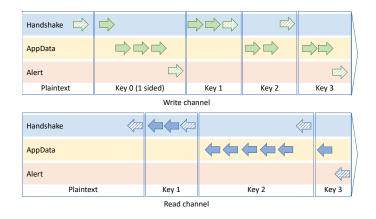
Figure 1: Multiplexing of sub-protocol streams by the record layer, depicting a TLS 1.3 0-RTT handshake with re-keying.
