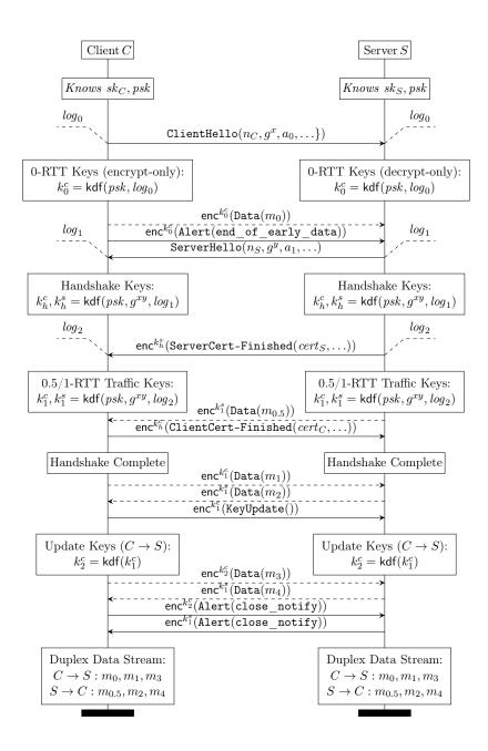
Figure 4: TLS 1.3 Draft-18 Protocol, seen from the viewpoint of the Record Protocol. Dotted arrows represent zero or more (encrypted) application data fragments. Each key stands for an instance of LHSE.
