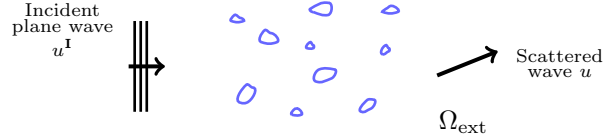
Figure 1: Scattering of a plane wave by various and non-overlapping obstacles. \Omega_{\text{ext}} is the domain outside the obstacles.
