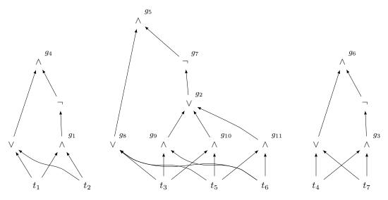
Figure 4: Boolean circuit for queries  $Q_1$  and  $Q_2$
