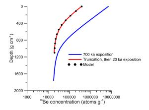
**Figure 6.** Illustration of "pseudo-inheritance". The plot shows a theoretical profile which was exposed for 700 kyr. Then 3 m were truncated immediately. Afterwards, the profile was again exposed to the cosmic radiation for 20 kyr. We modeled the age (31 kyr) and inheritance  $(19 \times 10^4 \text{ atoms g}^{-1})$  using excel.
