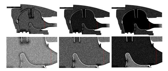
Figure 5: Top: increasing refinement of the mesh from 11 to 220 millions of elements. Bottom: detailed view
