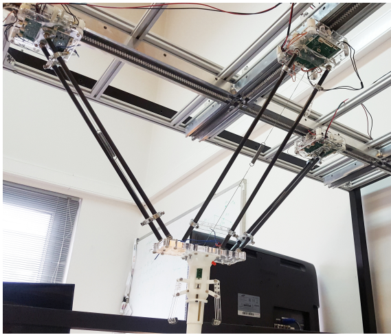
Fig. 12. PKM prototype developed at ISR-UC, using the design method proposed in this work.
