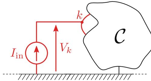
**Figure 1.** A partial transfer function of circuit  $C$  is determined by connecting a small-signal current source at node  $k$  and by determining the circuit's voltage response to this small-signal current excitation.
