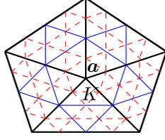
Figure 1: Example of nested meshes with  $J = 2$ . Coarsest mesh  $\mathcal{T}_0$  with  $\mathbf{a} \in \mathcal{V}_0$  and  $\omega_0^{\mathbf{a}}$  constituted by 5 elements (black, thick), first refined mesh  $\mathcal{T}_1$  (blue, thin), and second refined mesh  $\mathcal{T}_2 = \mathcal{T}_h$  (red, dashed).  $\mathbf{V}_{1,0}^{\mathbf{a}}$  consists of  $\mathbf{RT}_p$  functions associated with blue (thin) elements and edges that lie inside  $\omega_0^{\mathbf{a}}$ .
