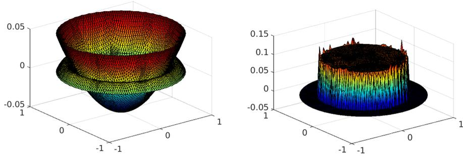
Figure 2: Solution at convergence for approximately 8000 elements. Left: position of the membranes ( $u_{1h}, u_{2h}$ ). Right: discrete action ( $\lambda_h$ ).
