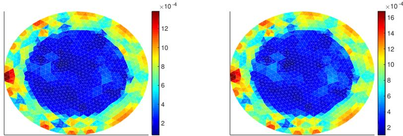
Figure 9: Error in energy norm (left) and total estimator (right), adaptive inexact Newton-min method,  $p = 1$ .
