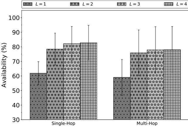
Figure 5: Comparing availability using NDN+CoCa in a single-broadcast vs a multi-hop scenario. Results for  $p = 0.95$ , uncoordinated sleeping and varying data lifetimes  $L$ . The cache can store up to 80 entries per node.
