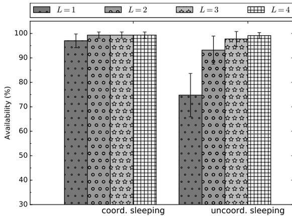
Figure 10: Comparing availability with NDN+CoCa using *coord.* or *uncoord. sleeping*, for different values of  $L$ . The interval of the active cycle was set to 30 s in the *coord. sleeping* approach and  $p = 0.8$  for the *uncoord.* one.
