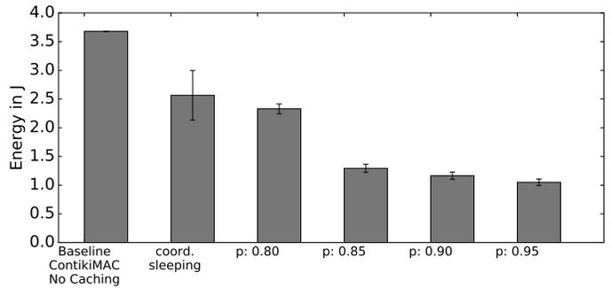
Figure 12: Older IoT hardware: Average energy consumption per node for *coord.* and *uncoord. sleeping* approaches on an MSP430 based node. ContikiMAC is used for RDC. Active MCU consumes 0.5 mA, listening consumes 19.9 mA and a broadcasts costs approx. 2.8 mJ.
