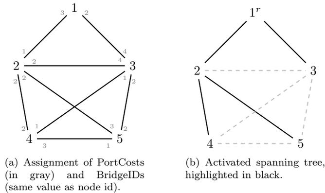
Figure 1: Example of PortCost and BridgeID assignment and resulting spanning tree. Node 1 is chosen as the Root Bridge. Even though path  $\{1,2,4\}$  and  $\{1,3,4\}$  have both length 8, the first is chosen because the BridgeID of node 2 is smaller than of node 4.
