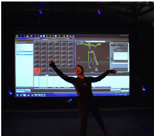
Figure 1. The data collection using EMGs, an accelerometer and a Vicon Motion Capture
