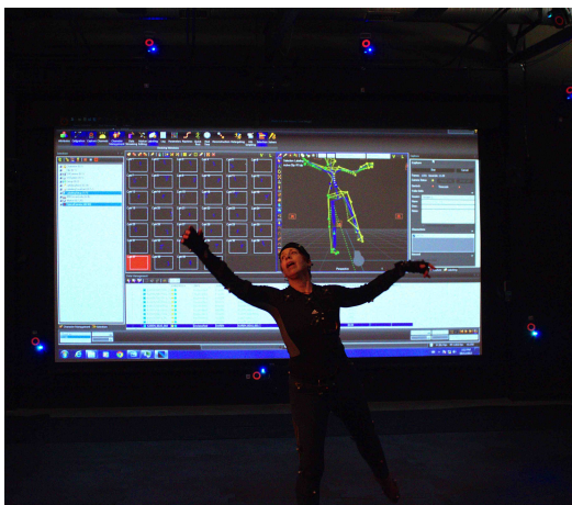
Figure 1. The data collection using EMGs, an accelerometer and a Vicon Motion Capture
