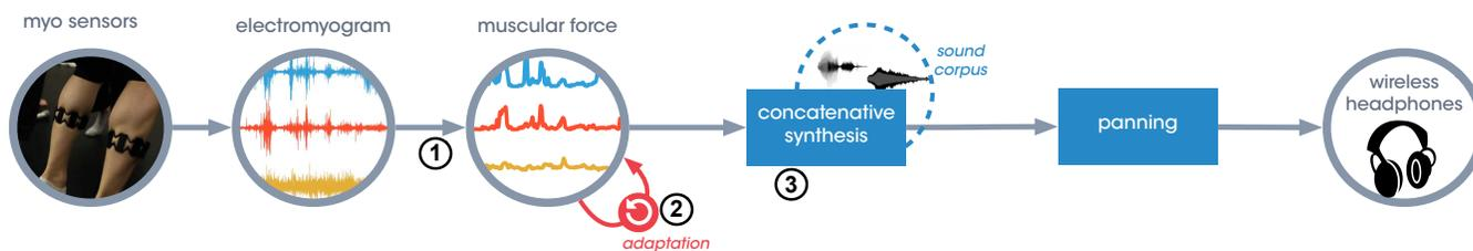
**Figure 3.** Synthetic architecture of the *still, moving* system. (1) the muscular activity is captured by EMG using Myo sensors, and the force is estimated using bayesian filtering. (2) The force is rescaled using on-line adaptation. (3) The force controls the concatenative synthesis of environmental sounds.
