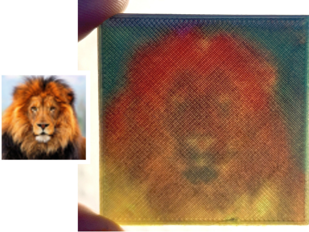
Fig. 18. A low-resolution lion image is used to drive a mixing field and produce a colorful lithophane (printed flat and backlit).
