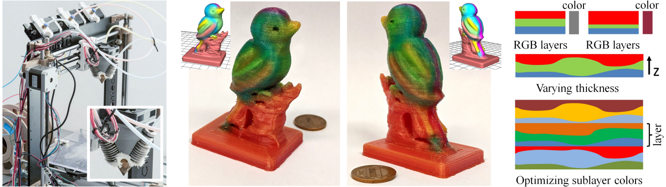
Fig. 1. Our technique enables color printing with precisely controlled gradients using a filament printer. Left: The printer is equipped with an off-the-shelf nozzle that inputs multiple filaments (three in the picture) and outputs molten mixed plastic through a single exit hole. Such devices cannot directly be used to print gradients: the transition between mixtures takes time, and this timing varies unpredictably. Middle: Using our technique, a user can 3D paint a virtual model and print an accurate, colored physical realization of her design. Printing uses standard, widely available materials (e.g. PLA, PET). Right: Our approach divides each layer into strata of varying heights to reproduce colors, printing them one on top of another. The color of each stratum is optimized to reduce visible stripes and print time.
