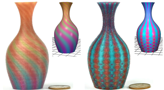
Fig. 17. 3D printed vases (Thing: 763726). Pictures of the print and 3D views in our paint tool in the insets, with matching viewpoints.
