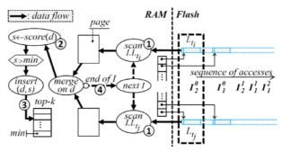
Fig. 4. Linear Pipeline computation of Q over terms  $t_i$  and  $t_i$ .
