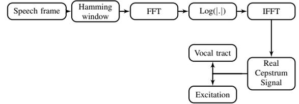
Figure 3: Bloc diagram of cepstrum based feature extraction
