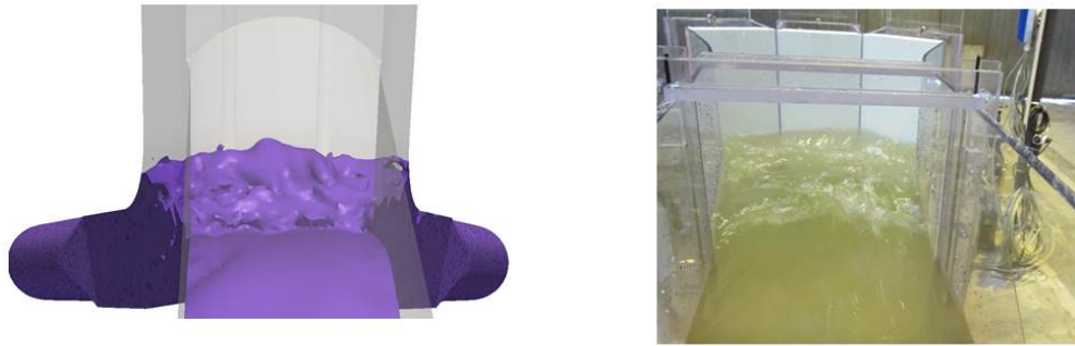
Figure 15 : Comparison between the numerical model (left picture) and the physical model (right picture). The drawn free surface is for \alpha = 0.5 .
