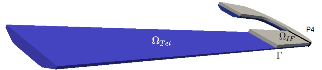
Figure 2 : Coupling geometry where \Omega_{Tel} and \Omega_{IF} are respectively Telemac-3D domain and InterFOAM domain, with \Gamma the coupling interface.
