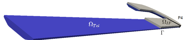
Figure 2 : Coupling geometry where \Omega_{Tel} and \Omega_{IF} are respectively Telemac-3D domain and InterFOAM domain, with \Gamma the coupling interface.
