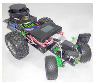
Fig. 7 Car with lidar and camera
