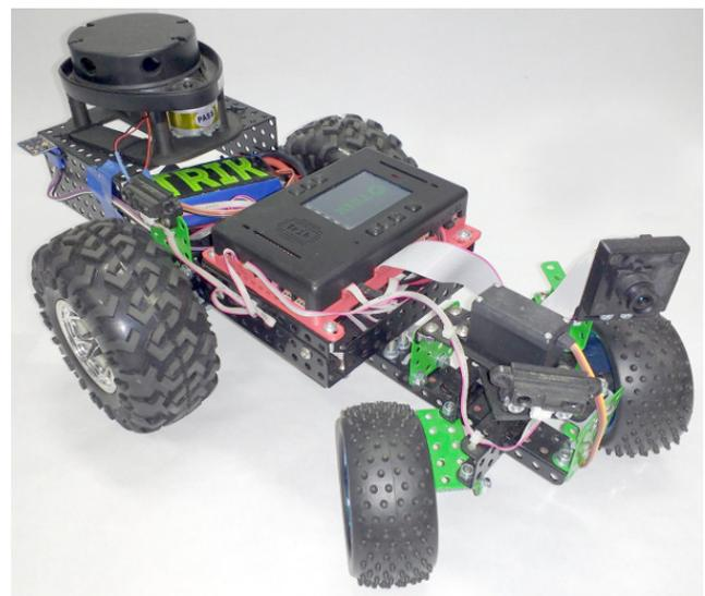
Fig. 7 Car with lidar and camera
