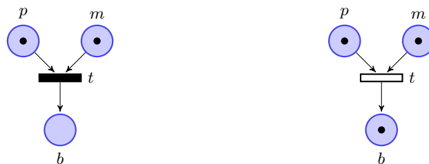
(a) Initial marking for the request \{p, m\} (b) Final marking for the request \{p, m\}
