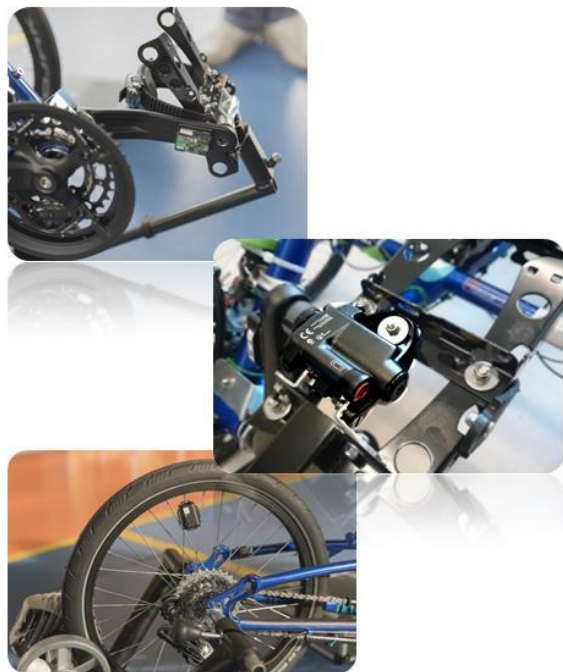
Fig 7. Power is computed via force pedals, cadence and speed are monitored via two inertial sensors (on the crank and rear wheel)
