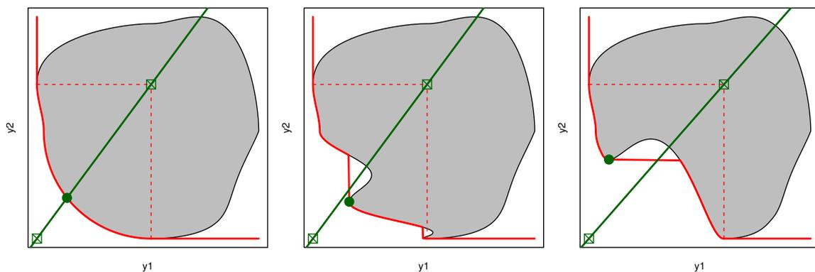
Figure 1: KS solution for a continuous (left) and discontinuous (center and right)  $\mathcal{P}^*$ . The KS is shown with a green disk, along with the shadow and nadir points (squares). The shaded area shows the feasible space, and the Pareto front is depicted in red.
