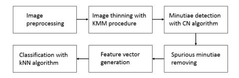
**Fig. 1.** Block diagram of fingerprint algorithm that was implemented in the application
