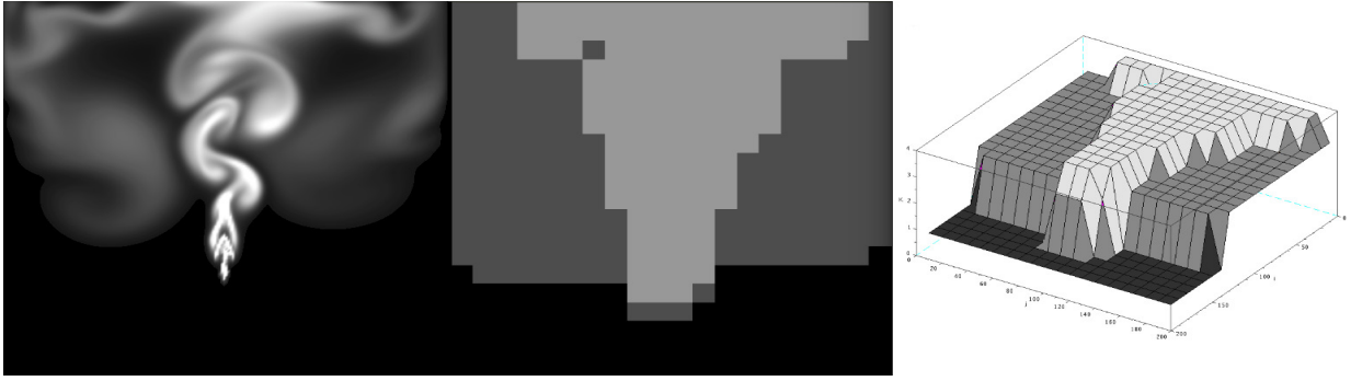
Fig. 3: Snapshot of the fluid simulation on the left, the corresponding grid state on the center and the volume of total computations (denoted by k ) on the right.
