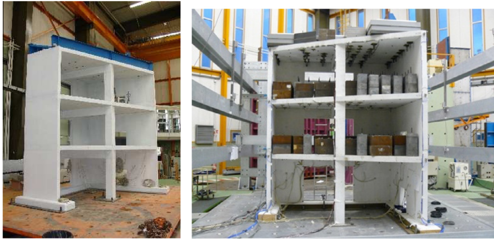
Fig. 5-7. Experimental SMART2008 mock-up. Left: bare specimen on shaking table; right: specimen on shaking table with additional masses during seismic test. © CEA/EMSL.
