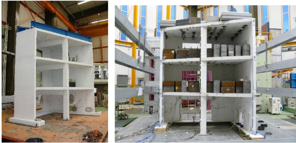
Fig. 5-7. Experimental SMART2008 mock-up. Left: bare specimen on shaking table; right: specimen on shaking table with additional masses during seismic test. © CEA/EMSI.
